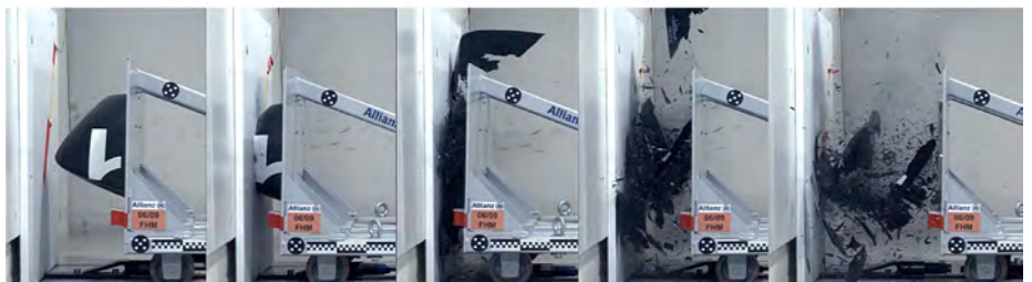
Crash test: Conventional structure
